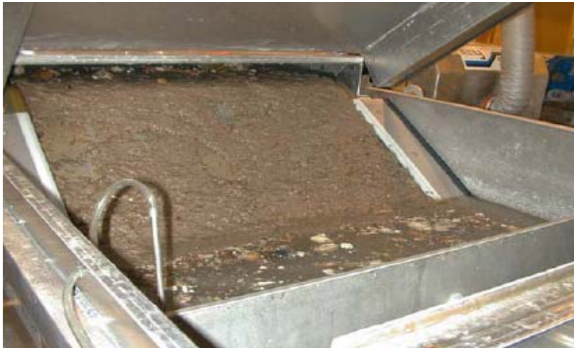
Figure 5-1 Salsnes Filter Wire Cloth
