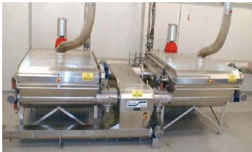
Figure 5-2 Parallel Salsnes Filters
